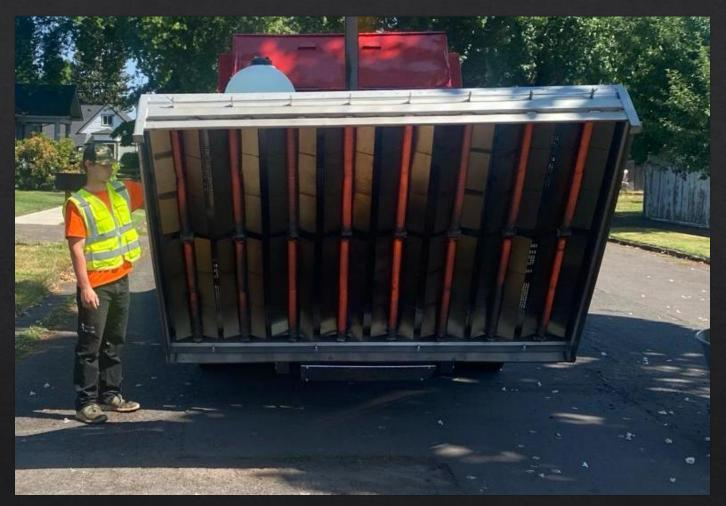
The chamber is hydraulically operated on our truck and trailer mount units – no cables or winches are used on Kasi machines ensuring safety.
